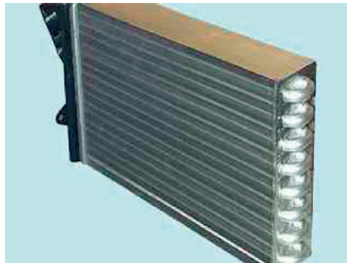
Figure 2.162 The heater matrix (radiator) is similar to the main radiator but smaller
